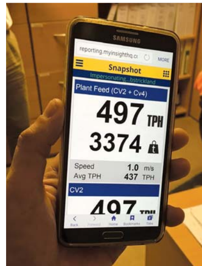
FAR LEFT: InsightHQ is fitted on Shap Beck's Volvo L220 and L250 wheeled loaders LEFT: Limestone products come off the conveyor onto a stockpile at Shap Beck quarry BELOW: Updated every minute, InsightHQ's Snapshot tool can offer instant quarry site performance data
