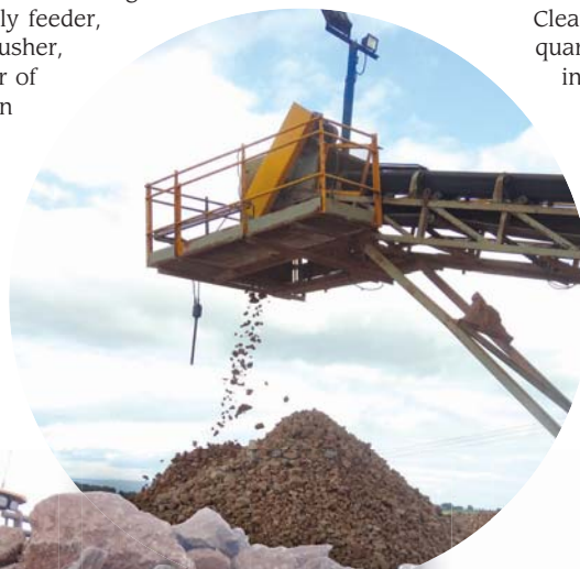
FAR LEFT: InsightHQ is fitted on Shap Beck's Volvo L220 and L250 wheeled loaders LEFT: Limestone products come off the conveyor onto a stockpile at Shap Beck quarry BELOW: Updated every minute, InsightHQ's Snapshot tool can offer instant quarry site performance data
