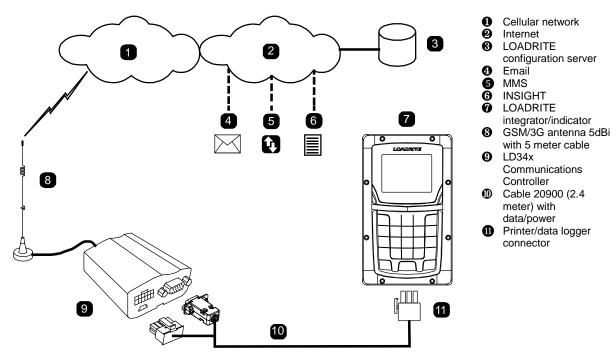
The LCC uses cellular networks to transmit data. Consult your local cellular provider to ensure compatibility.
