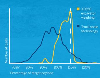
Haul truck payload measurement systems are useful but only provide suitable information after the truck has left the load out location. The driver must then either accept an under or overload, or return to the face to dump the load. All of which compromise productivity.
